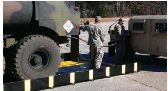
Fail-Safe® MilBerm™ safely captures leaks or spills during refueling operations.
