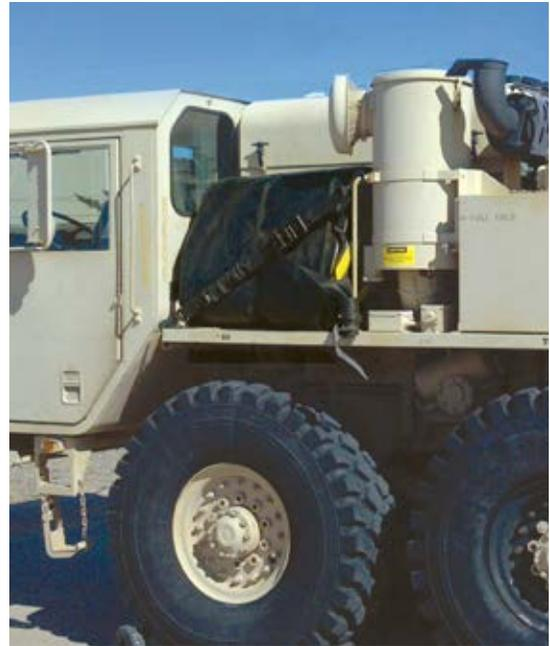
Folded Fail-Safe® MilBerm™ securely attached to the HEMTT tanker for deployment at a moment's notice.
